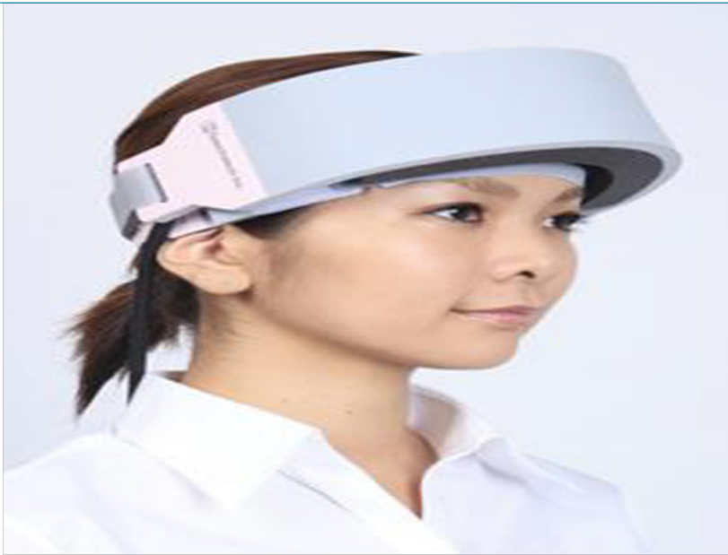
Figure 1 -flow of the blood at the frontal part of the brain was measured using 16-channel optical encephalography using the OEG-APD series instrument developed for encephalography
